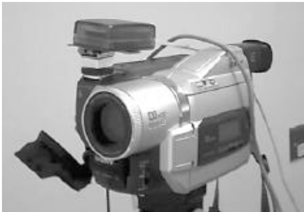
Figure 2. Digital video camera with GPS receiver attached at top determines viewer location, direction of view and focal length. Smaller laptop-mounted cameras have since been used to minimize weight and inconvenience.
