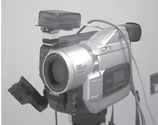
Figure 2. Digital video camera with GPS receiver attached at top determines viewer location, direction of view and focal length. Smaller laptop-mounted cameras have since been used to minimize weight and inconvenience
