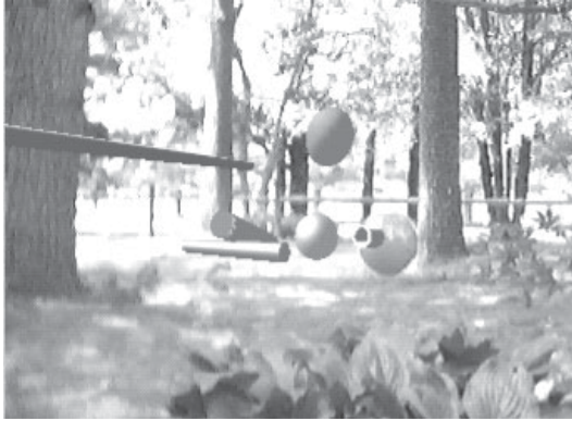
Figure 8. An initial sketch using AmbiViewer. The bottom ball on the right is the fiduciary marker for the mixed reality. The rest of the balls, cylinders and hovering bar are simulations
