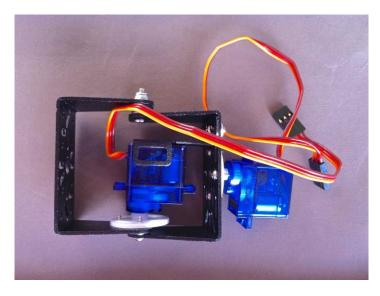
Figure 5. Motorized pan-tilt bracket.
