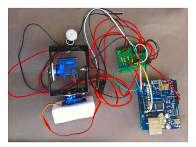
Figure 11. Finished lighting unit
