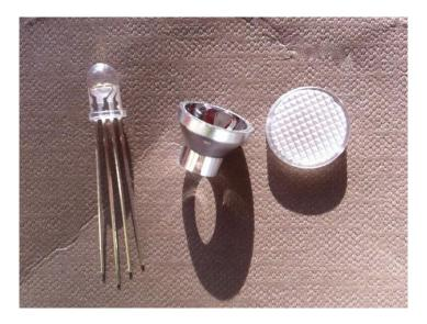
Figure 2. RGB-LED, reflector and diffusor.
