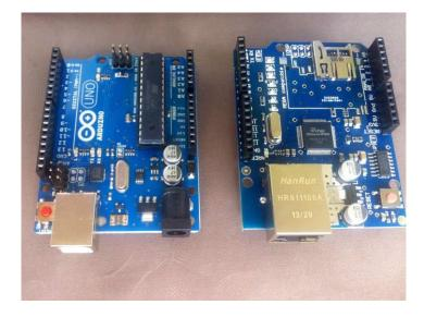
Figure 7. Micro-controller board and Ethernet shield
